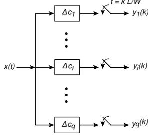
**Fig. 1.** Multi-coreset sampler implemented as a multi-channel system.
